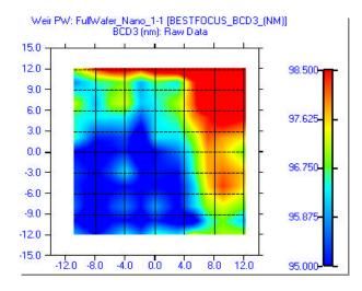
Figure 3: Bottom CD (BCD) average field from wafer scatterometer measurements.
