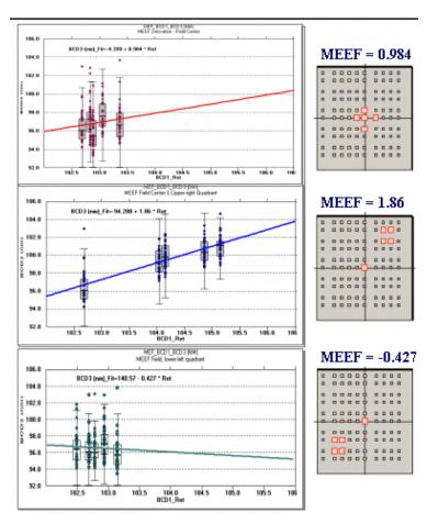
Variation in MEEF local calculation across exposure field. Figure 2a (top): MEEF calculated for five sites in the center of exposure field.
