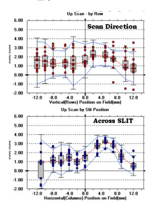
Figure 8A: MEEF variation along reticle SCAN Figure 8B: MEEF variation across the Lens Slit
