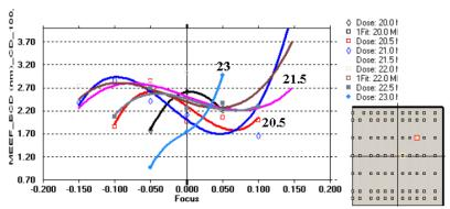
Figure 11: MEEF Response to Focus for one site, shown as highlighted site in the inset on the right.
