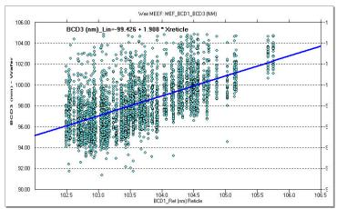
Figure 1: MEEF=1.9018 calculated from the measured Bottom CD (BCD) size in the resist and the Reticle feature size (BCD1 Ret) at final size.
