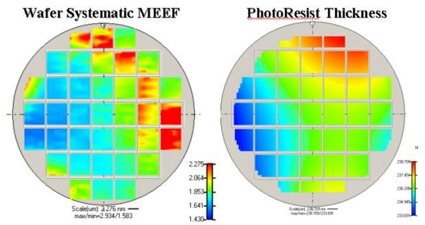
Figure 10: MEEF response to resist thickness.
