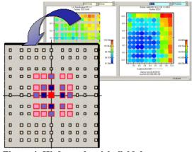
Figure 4: Wafer and reticle field datasets are analyzed using an Adaptive Floating Kernel for localized MEEF calculation.
